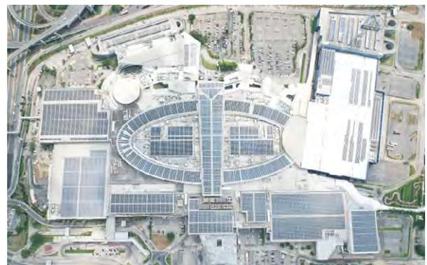
The solar power system for Mega Bangna is installed on the roof of the Mega Bangna shopping mall, covering an area of 60,000 square meters. It has a capacity of 9.89 MW, which can reduce greenhouse gas emissions and electricity costs, saving over 1.04 Billion Baht over the project’s 25-year lifespan.
